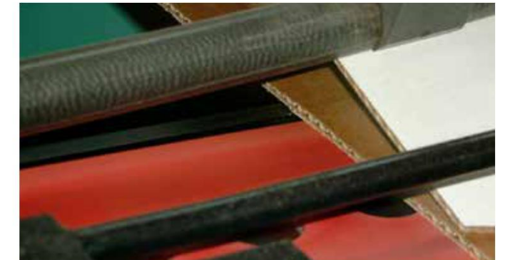
Flexo Folder Many producers use P6-type (rough top) PVC or rubber surface coatings where the structure wears off rather quickly and varies the friction of the belt against the box. Natural rubber is our solution to avoid jamming and skewing.
