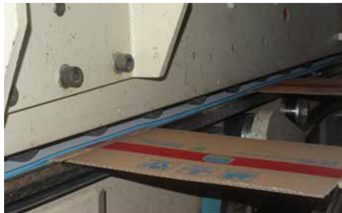
Excellent carton grip and increased output thanks to wear resistant XNBR Elastomer cover with P6 structure.
